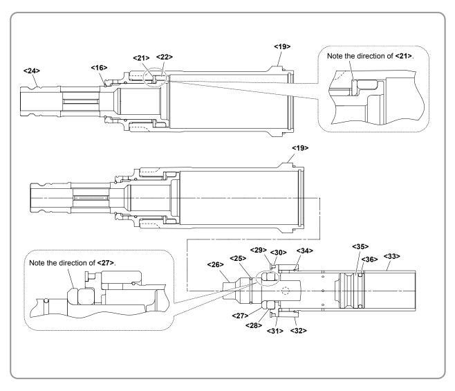
(4) Reassembly of the vibration reduciton mechanism (Model H 45MEY only):
